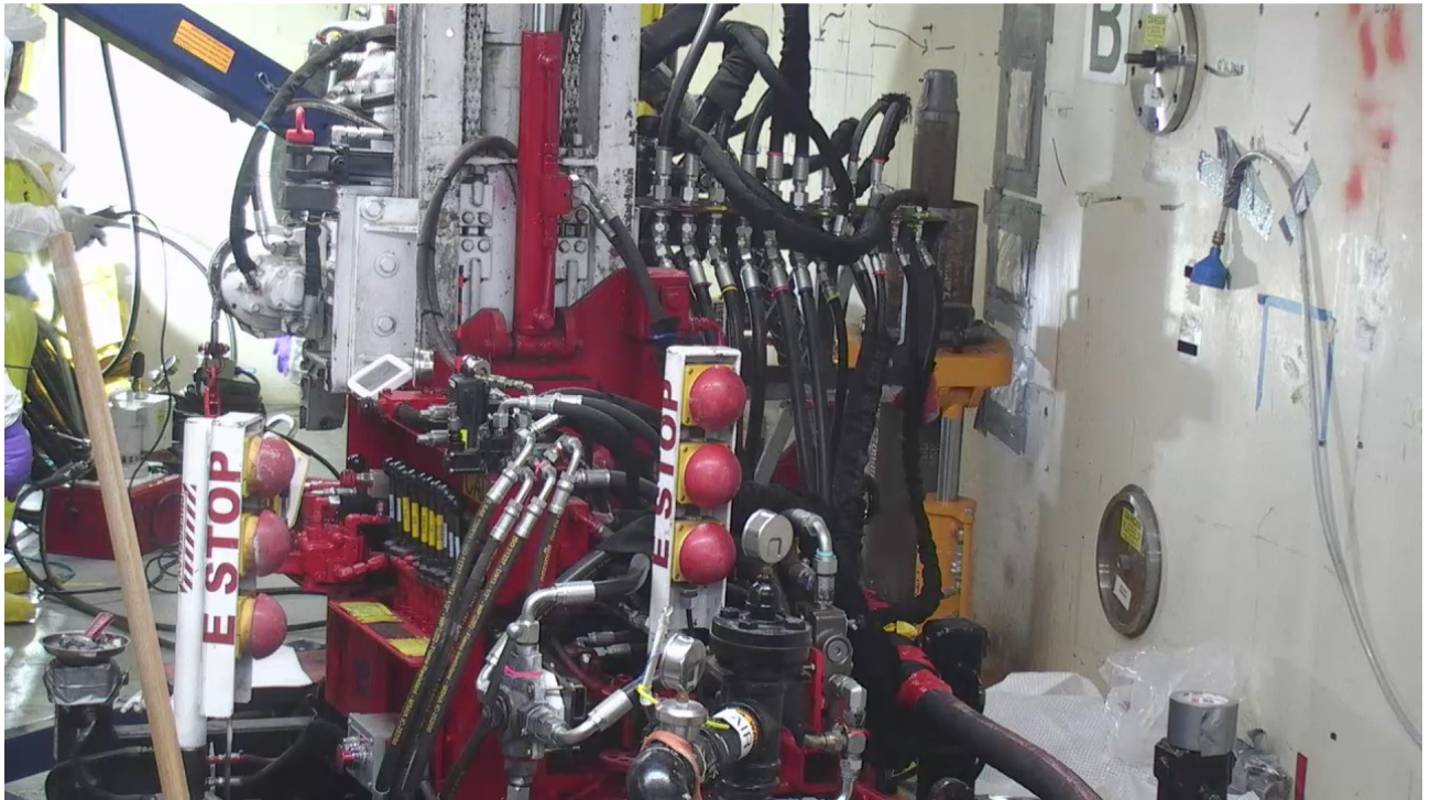
Jacks backpulling casing from borehole
