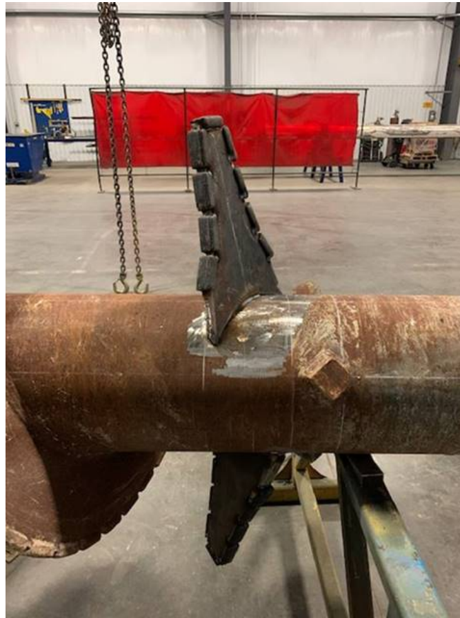
Temporary placement of knockdown paddle on VPC Auger Tool
