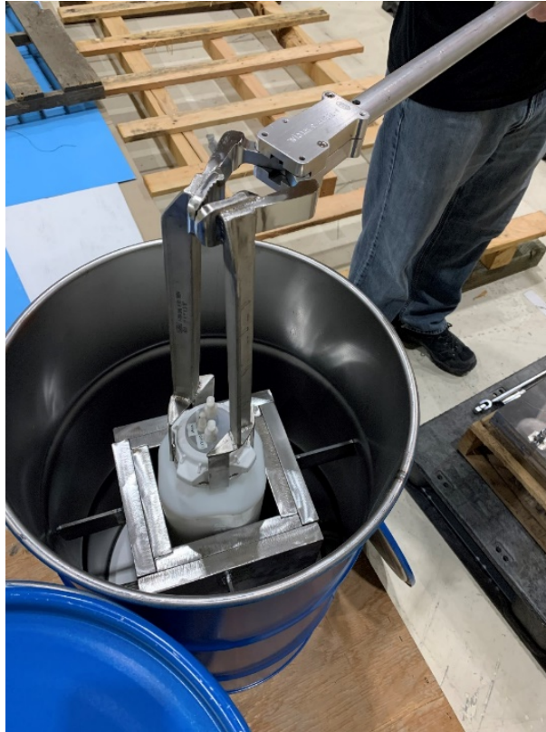
Operator familiarization with sample bottles, bottle handling tool, and shielded drum
