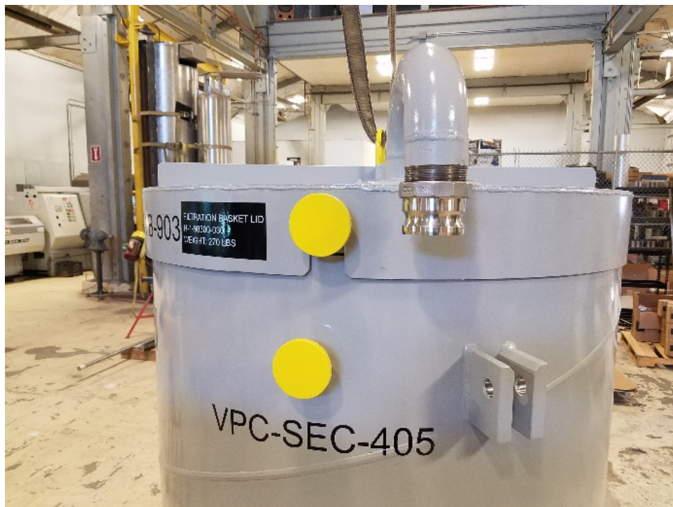
Filter Basket Assembly (top piece in photo) fit up test with VPC Debris Section
