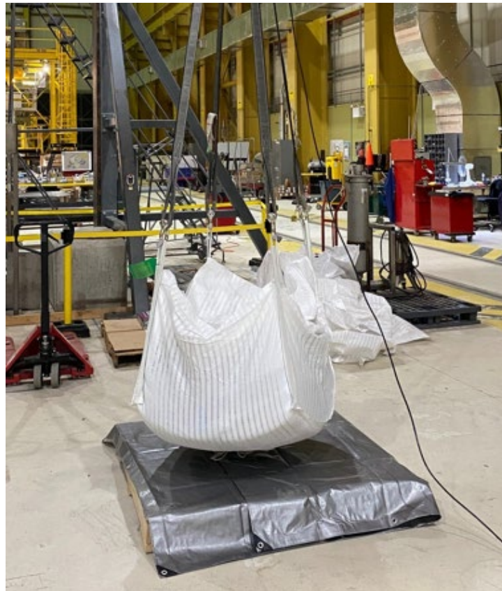
Modified Zeolite Filter Bag Load Testing
