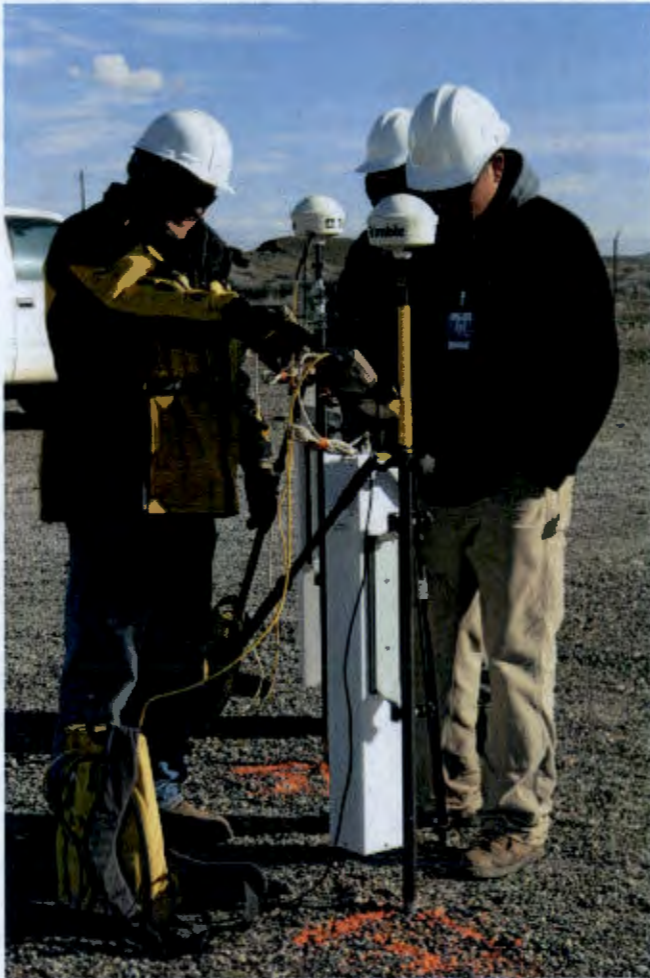
Figure 3.2 Reoccupying the Base Station to Calibrate the Instruments
