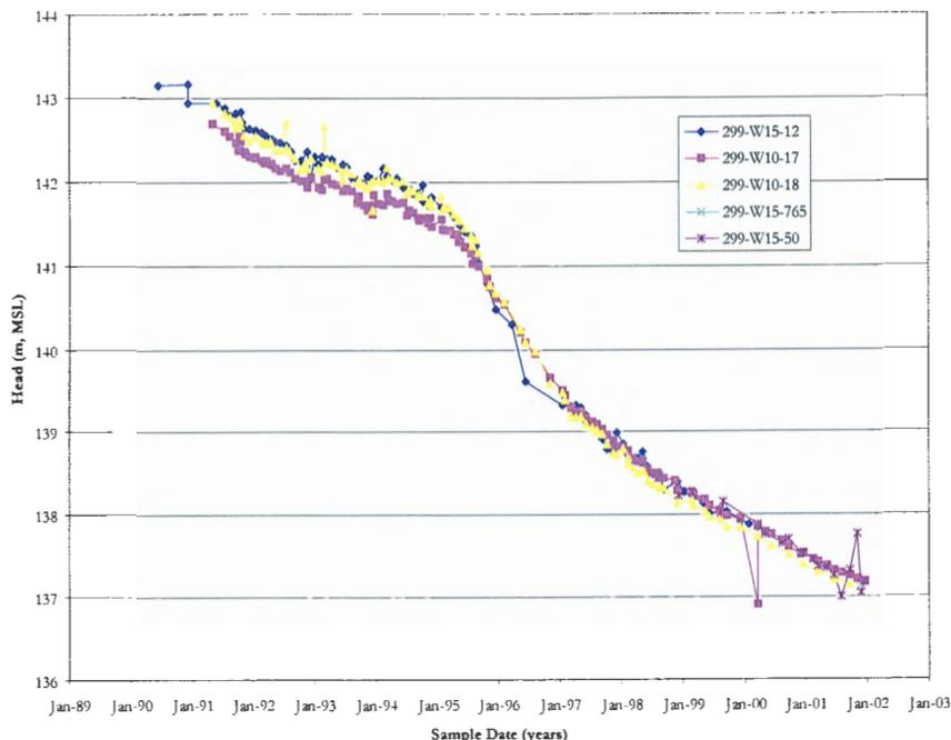
**Figure 4.18.** Water-Table Elevations in Four Wells at the Northern Part of Waste Management Area TX-TY
