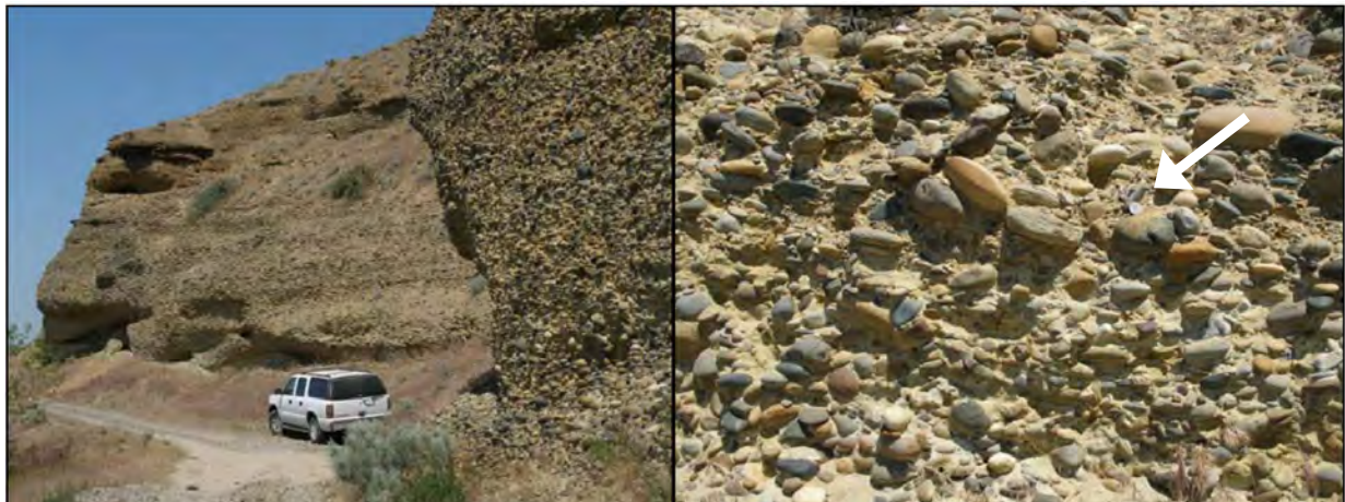
Figure 4.12. Ringold Formation Unit E conglomerate (member of Wooded Island [Lindsey 1995]) exposed near river level along the White Bluffs within 1 mile of the IFRC. Left: In the outcrop, these clast-supported, bimodal deposits may be crudely stratified and weakly imbricated, with occasional lenses of well-sorted fine- to medium-grained sand. Right: Light-colored pebble- to cobble-size clasts are mostly quartzite, granite, and gneiss; dark clasts are dominantly basalt, andesite, and volcanic porphyry (Campbell 1983). Note quarter for scale. Unlike the IFRC site, the Ringold Unit E in these outcrops has undergone chemical oxidation as indicated by a pervasive yellow-to brown iron-oxide stain, which coats all sedimentary particles. The vertical nature of the exposures signifies the semiconsolidated nature of these compacted and cemented sediments.
