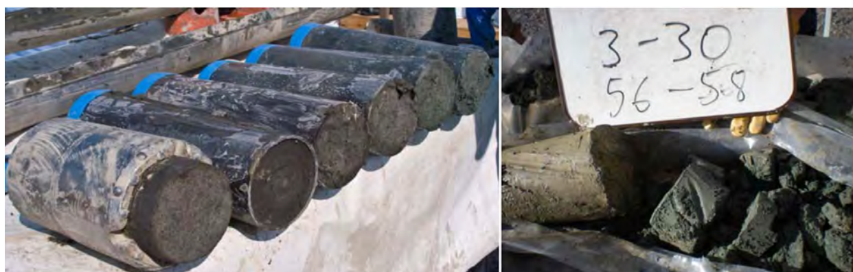
Figure 4.13. Fine-grained strata at the top of the Ringold Formation. Left: core samples collected from 59.5- to 65-ft depth in reduced silts and fine sands of the Ringold Formation in well 399-2-25. Top of the core is to the upper right. Right: Sharp contact exists between oxidized pale-brown (left) and reduced dark greenish-gray (right) silt layers in well 399-3-30 at the 57-ft depth. Top of the core is to the left.
