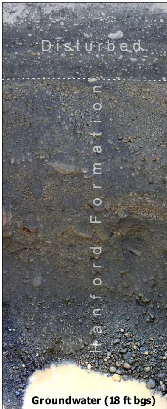
Figure 2.4. Vadose-zone backhoe pit SPP#2 excavated beneath the IFRC site in 2003. The uppermost 4 ft of the profile lack primary sedimentary structure, apparently destroyed from movement of heavy equipment over the site during remediation. Photo from Bjornstad (2004).
