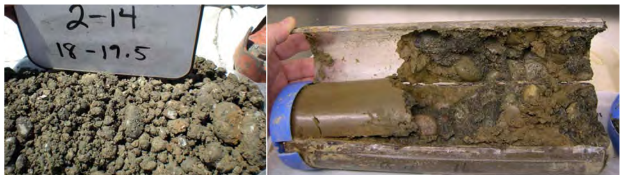
Figure 4.24. Flood gravels with fine-grained, reworked Ringold Formation matrix in the Hanford formation. Left: Matrix of olive to yellow Ringold Formation silt may be derived from erosion beneath the IFRC site or upstream off the White Bluffs. Grab sample from well 399-2-14, 18- to 19.5-ft depth. Right: The matrix surrounding clast-supported gravel in this core consists of a mottled mixture of multi-genetic brown Ringold Formation silt and dark gray basaltic sand (well 399-2-25, 52-ft depth).
