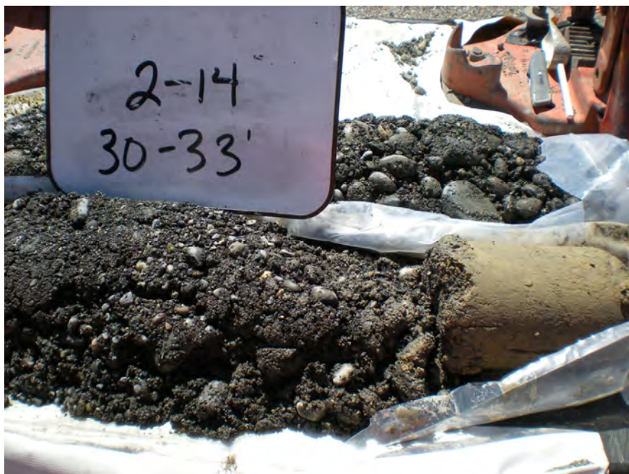
Figure 4.29. Loose, basaltic pebbly sand overlies the top of a semiconsolidated Ringold Formation rip-up clast within the Hanford formation at 30- to 33-ft depth, well 399-2-14. This rip-up clast is similar to the oxidized silt of the Ringold Formation that directly underlies the IFRC site.
