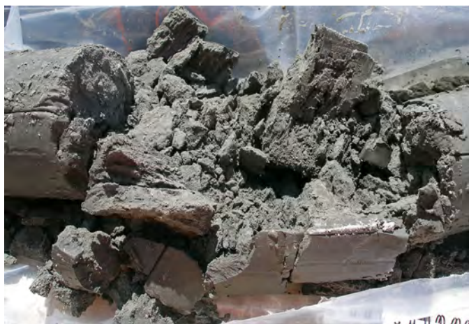
Figure 4.9. The Ringold lower mud unit at 160-ft depth in well 399-2-25 is predominantly a compact, homogeneous, dark greenish-gray, weakly stratified, fine sandy silt.
