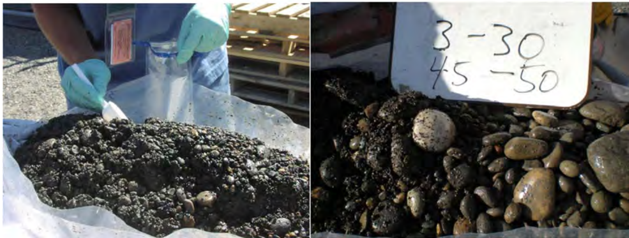
Figure 4.23. Gravel-dominated facies with openwork fabric within the Hanford formation. Left: Grab sample of loose, basaltic, pebble gravel was collected for microbiological characterization. Right: Clean, matrix-free pebble gravel on the right transitions to sandy, matrix-filled gravel to the left.
