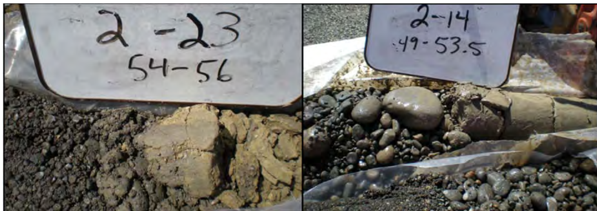
Figure 4.22. Sharp contact at the top of the Ringold Formation silt-dominated sediment in well 399-2-23 (left) and 399-2-14 (right). Notice the loose gravel in right-hand photo has little or no matrix.
