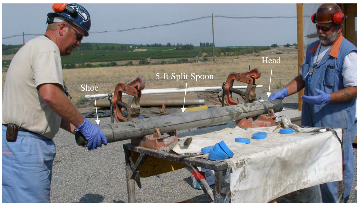
Figure 3.6. Sediment-filled split-spoon sampler. Notice cohesive Ringold Formation core protruding from shoe. Sediment core naturally expanded upon release of highly compressive drilling stresses.
