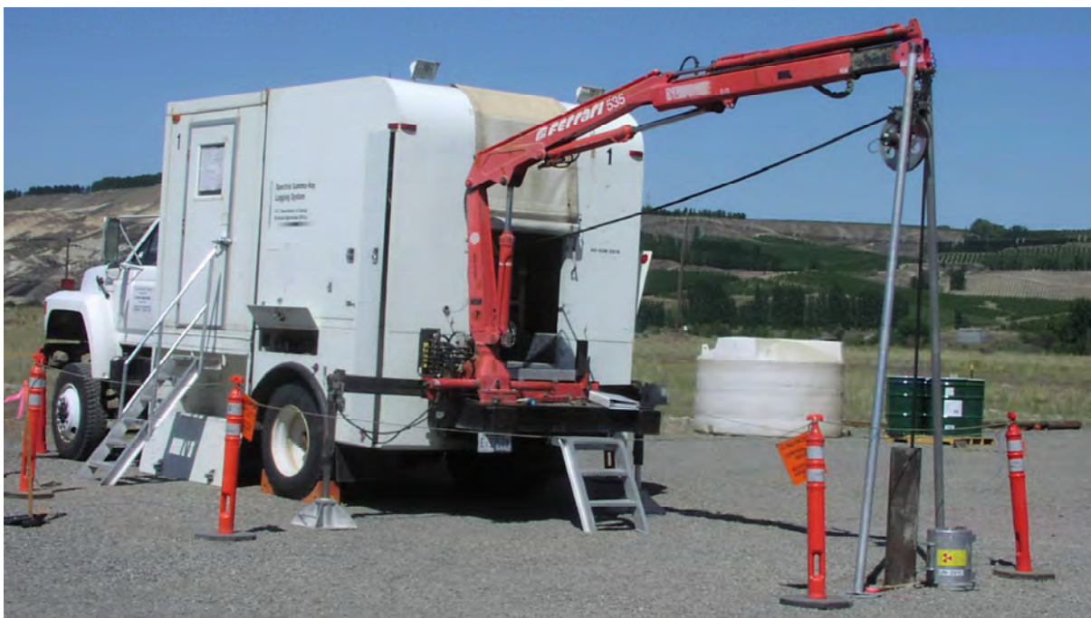
Figure 3.11. Downhole geophysical logging was accomplished through the temporary 7-5/8-in. (OD) steel casing via Stoller's spectral-gamma logging system.
