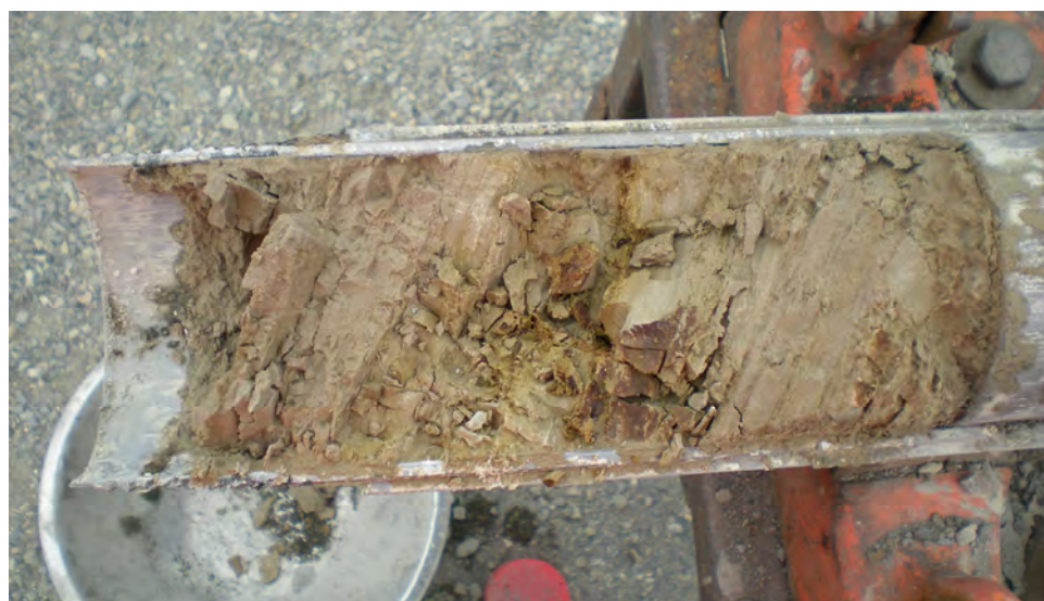
Figure 4.30. Portion of a 5.5-ft-thick semiconsolidated Ringold Formation rip-up clast, composed of cohesive clayey silt, in well 399-3-26 from 21- to 22-ft depth. The inclined lamination in this vertical drill core indicates this sediment was not deposited in situ but rotated in transit and redeposited during an Ice Age flood.
