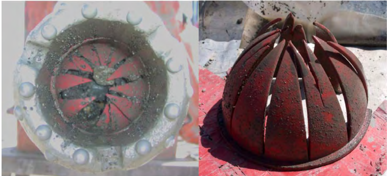
Figure 3.10. A plastic core catcher helped to keep loose Hanford formation sediments from falling out of the split spoon during core sampling.
