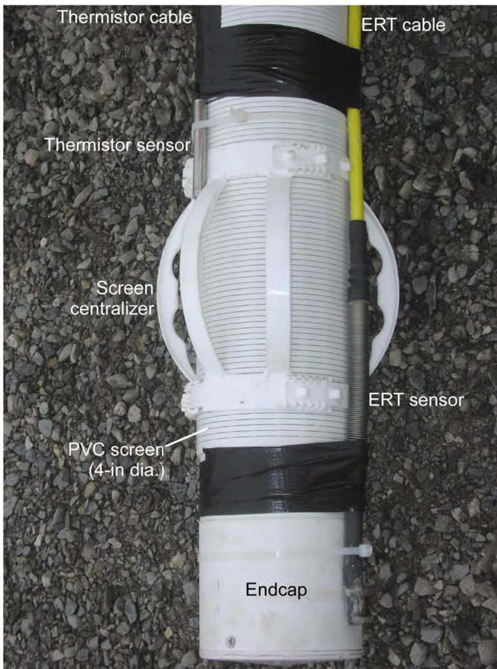
Figure 3.12. ERT electrode and thermistor sensors and cables were affixed at regular intervals down the outside of the 4-in. PVC screen and casing. A centralizer (shown) placed at the top and bottom of the screen kept the screen centered within the well and prevented it from coming into direct contact with the formation.
