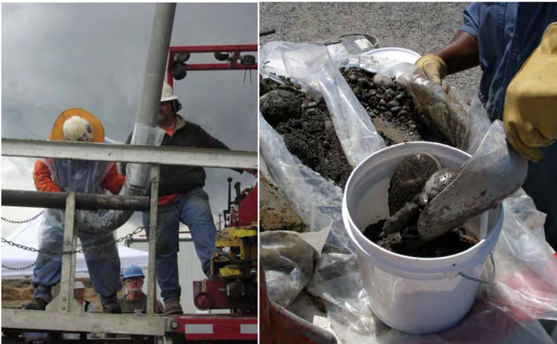
Figure 3.8. Bulk core and grab samples were collected from all IFRC wells not sampled via split spoon. Sediment core (left) was extruded via sonic vibration out of the core barrel into a knotted plastic sleeve. For grab-sample collection (right), core was transferred from the plastic sleeve into labeled 2-gal plastic buckets. Each bucket held 2 to 3 ft of core.
