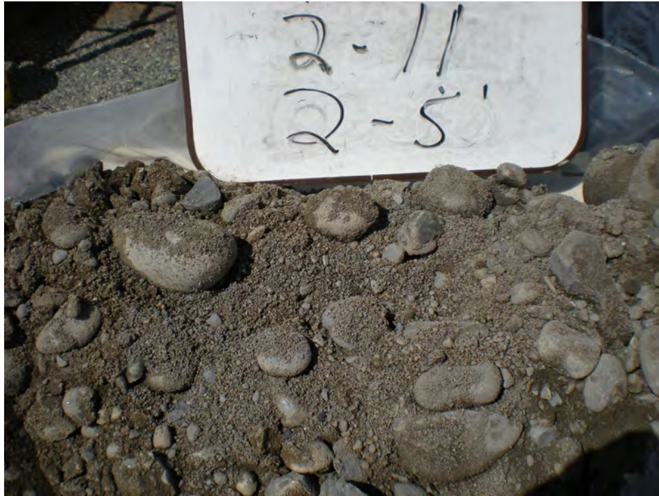
Figure 4.32. Backfill materials from 2- to 5-ft depth in well 399-2-11. This material is very similar to that of the Hanford formation from which it is derived. However, backfill sediments are likely more isotropic than the Hanford formation because the sedimentary fabric (horizontal to subhorizontal layering and stratification) was destroyed during excavation and backfilling.
