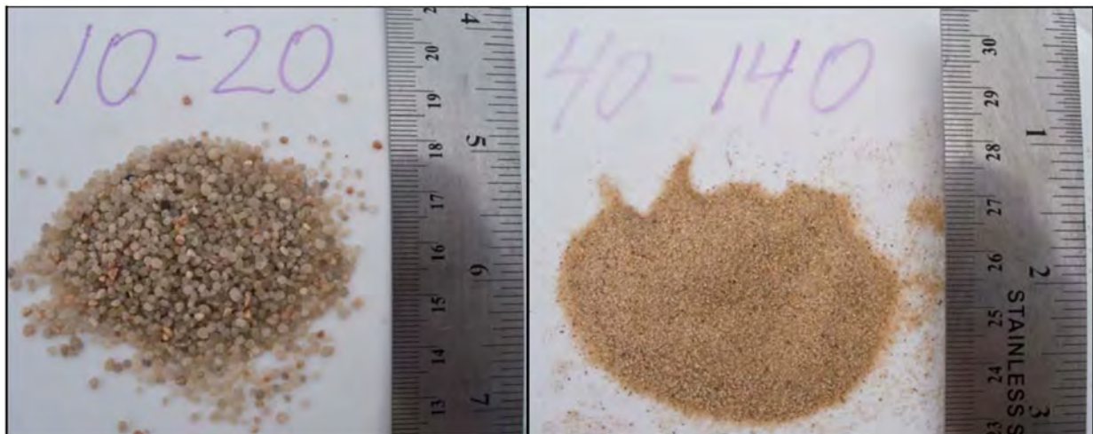
Figure 3.14. Comparison between coarser 10-20 mesh silica sand (left), used around 20-slot well screens, and the finer 40-140 mesh sand placed in the annular space above the screen
