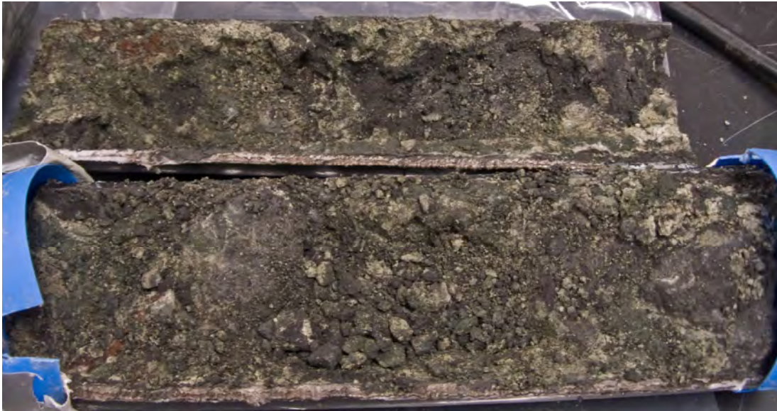
Figure 4.8. Core segment, weathered basalt of the Ice Harbor Member, from the bottom of well 399-2-25. The 1-ft-long Lexan-lined core consists of irregular fragments of black vesicular basalt in a highly weathered and green-gray mottled alteration-clay matrix. Light-colored material effervesces in contact with dilute hydrochloric acid, indicating the presence of calcium carbonate.
