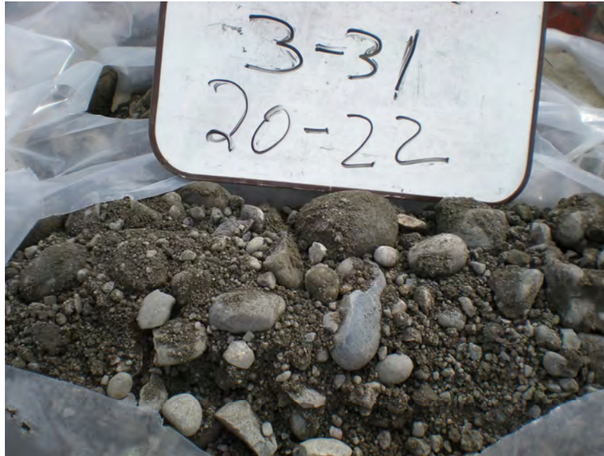
Figure 4.17. Typical appearance of gravel-dominated facies of the Hanford formation within the 300 Area. The sediment is loose, composed of brownish-gray, clast-supported, poorly sorted, silty, sandy, pebble-cobble gravel. Clasts are mostly subangular to subrounded basalt; other clasts include granitics, gneiss, and quartzite as well as other volcanics. Some of the larger clasts were broken apart during sonic drilling, whereas most smaller clasts are unbroken, an indication that the sonic drilling method produces relatively representative samples for characterization. This grab sample was collected from the 20- to 22-ft depth in borehole 399-3-31.
