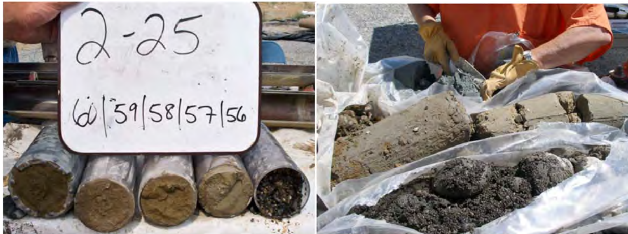
Figure 4.21. Hanford–Ringold formations contact. Left: Contact lies between coarse basaltic sand and gravel in right-hand core and next core, composed of oxidized Ringold Formation silt at the 57-ft depth (well 399-2-25). Right: Loose, basaltic sand and gravel of the Hanford formation (foreground) overlie oxidized (middle) and reduced (background) greenish-gray silt of the Ringold Formation (well 399-3-28).
