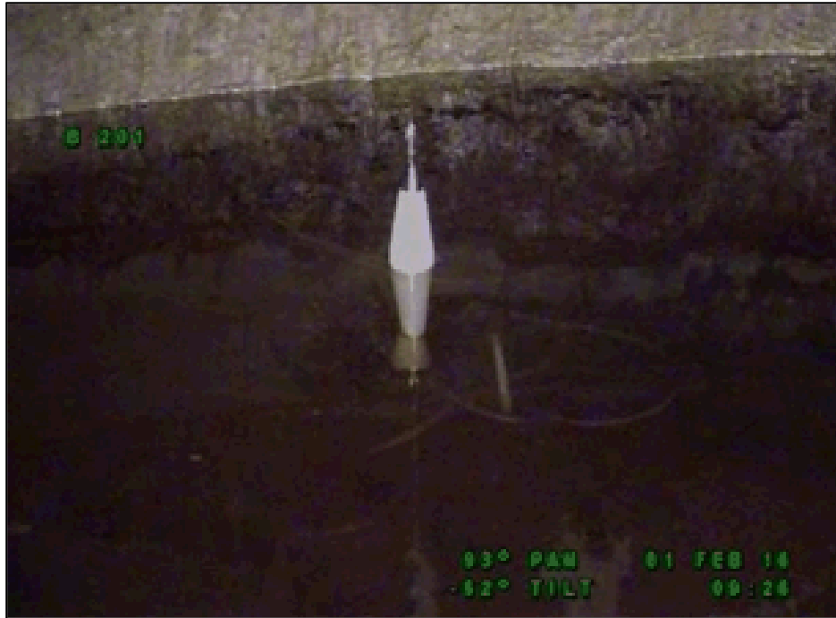
Figure 4. Enraf Plummet on Liquid Waste Surface.
