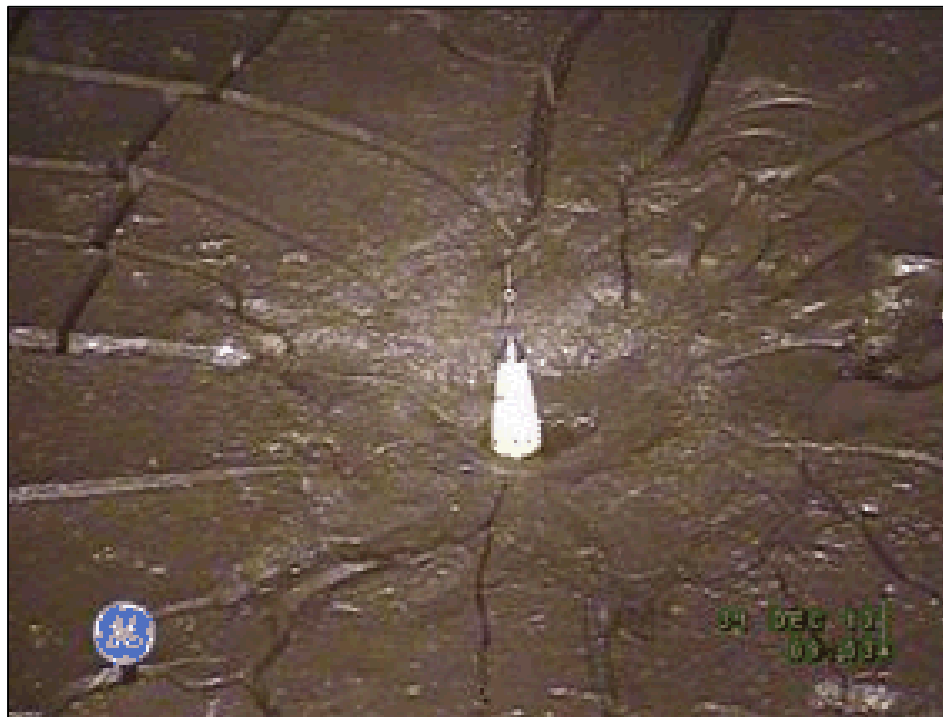
Figure 5. Enraf Plummet on Liquid Pool on Solid Waste Surface.
