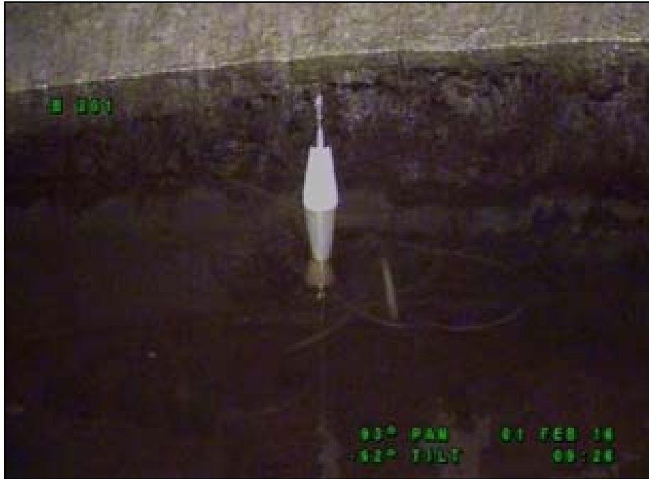
Figure 4. Enraf Plummet on Liquid Waste Surface.
