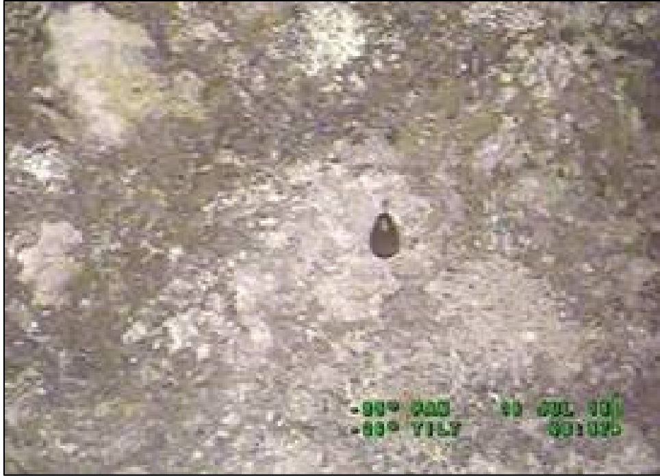
Figure 6. Enraf Plummet on Solid Waste Surface.
