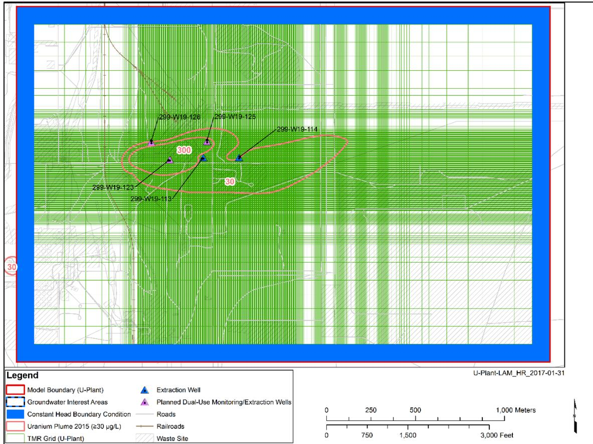
Figure 4. Horizontal Numerical Grid Discretization for the U Plant Submodel
