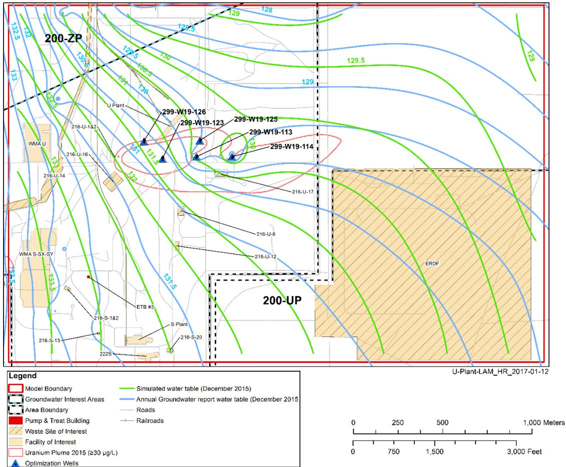
Figure 17. Comparison of Simulated and Mapped Water Table, December 2015
