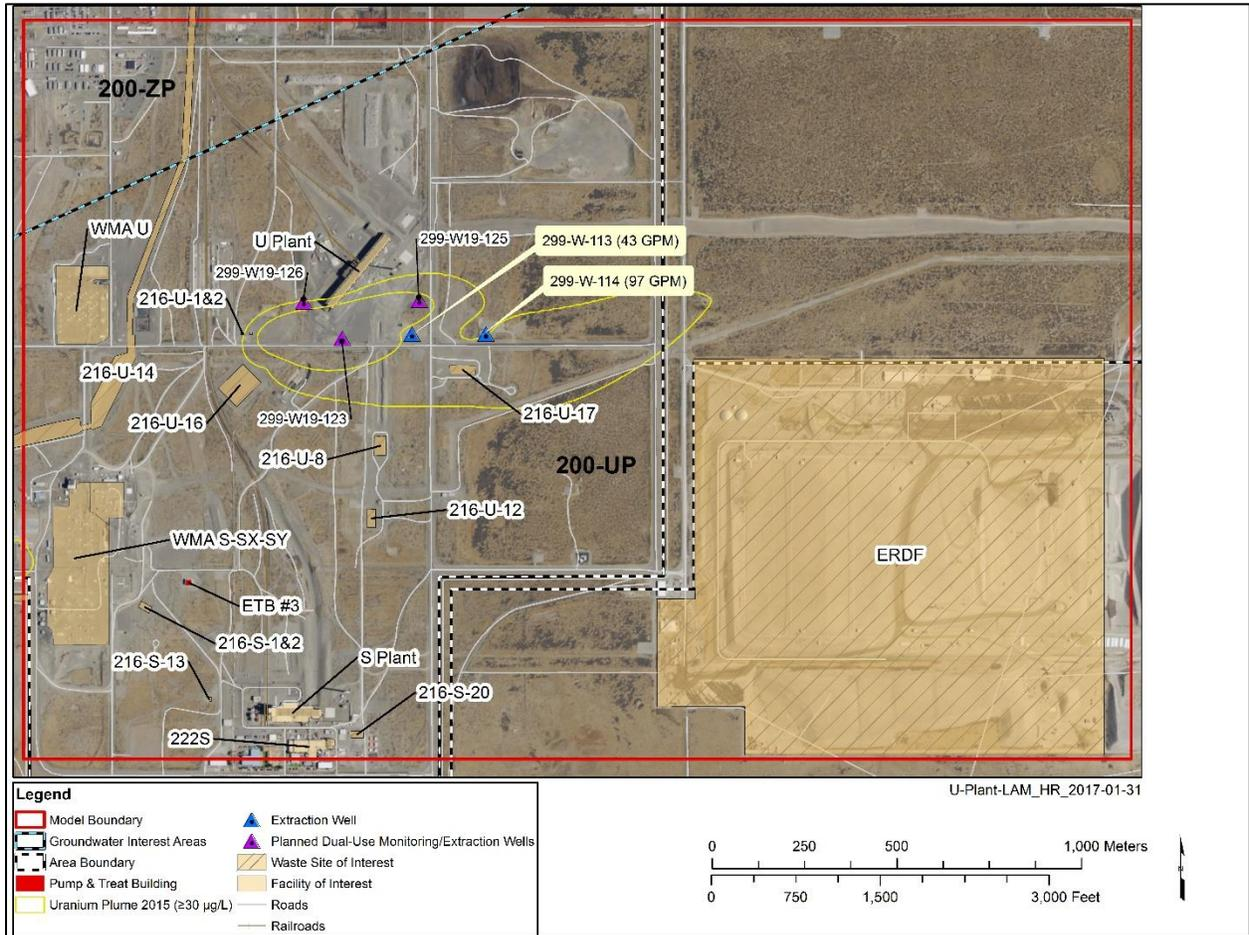
Figure 6. Extraction Well Locations and Fall 2016 Pumping Rates
