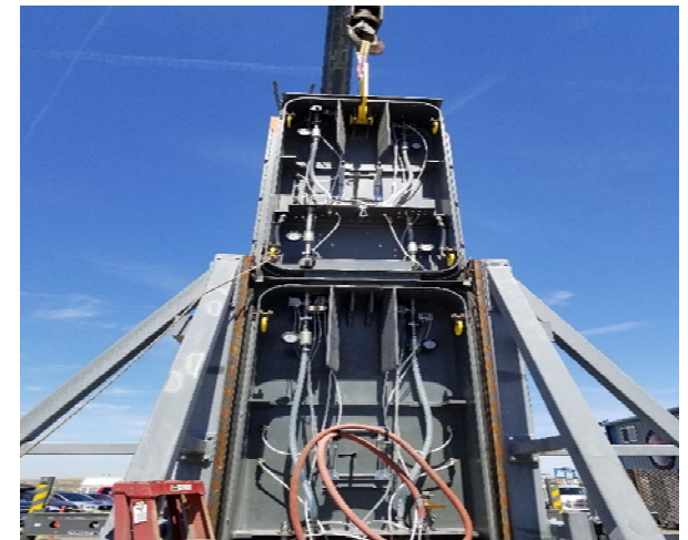
A Cell Mid Dam placed on top of the Lower Dam in the test stand at Hi Line Fabricating as part of the Factory Acceptance Test.
