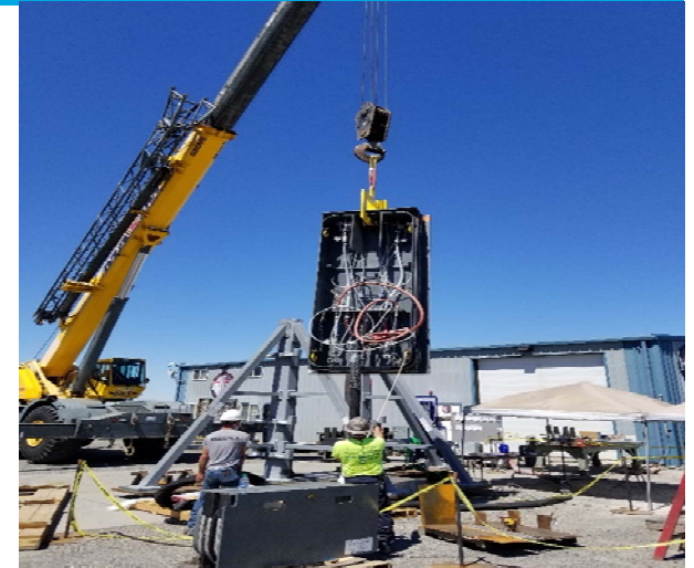
A Cell lower Dam being lifted into the test frame as part of the Factory Acceptance Test.
