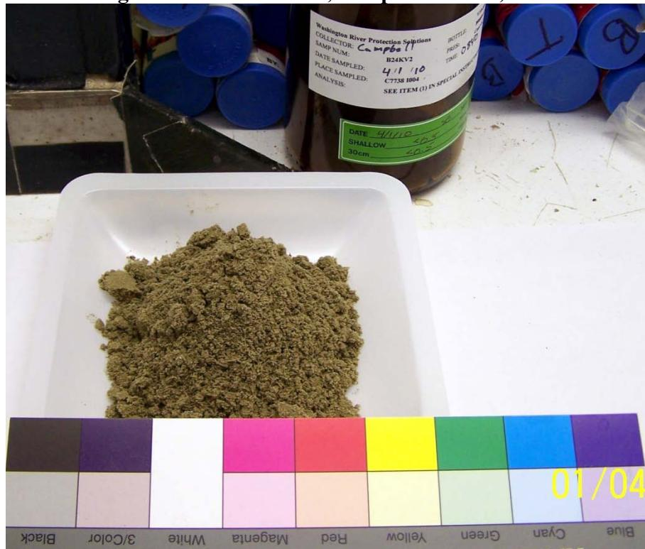
**Figure A-20: Core 7738, Sample B24KV2, Composite**
