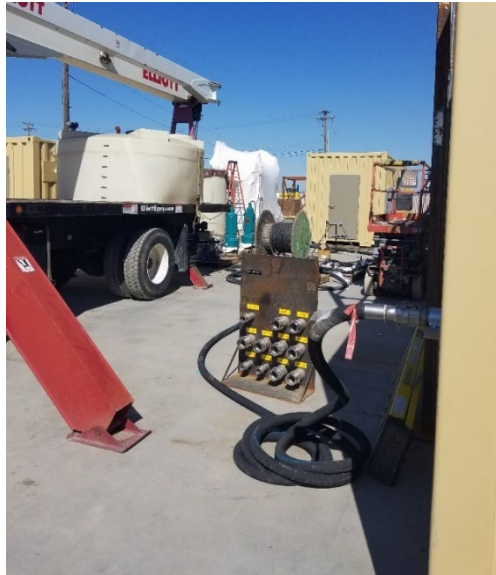
Testing the Dewatering Wall Pass-Thru
