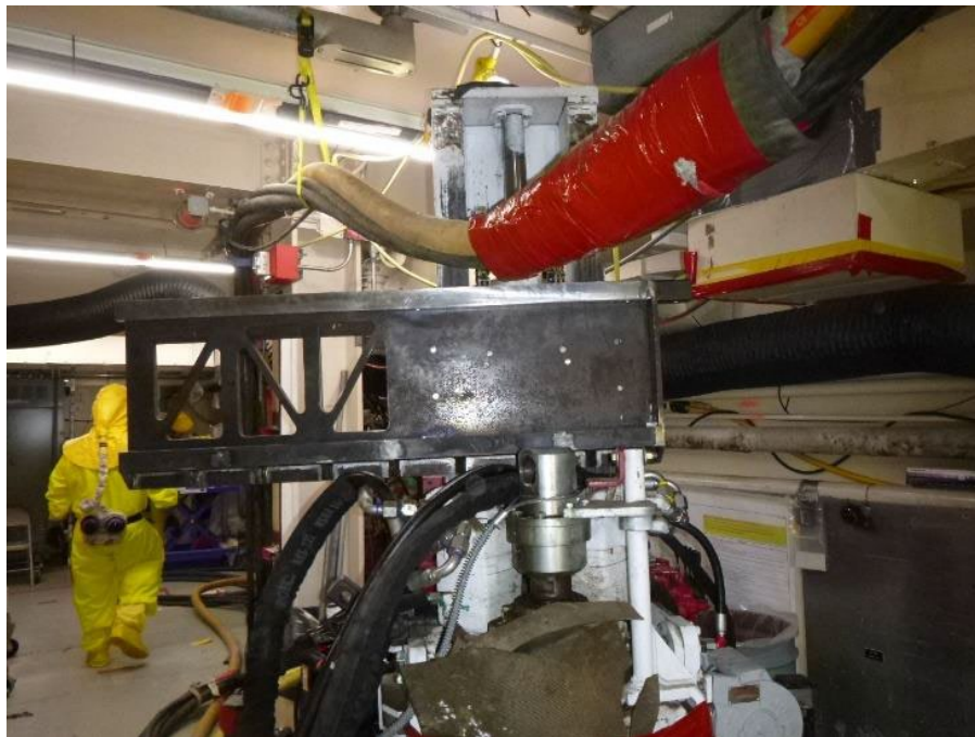
Head Slide installed on Room 18 Drill
