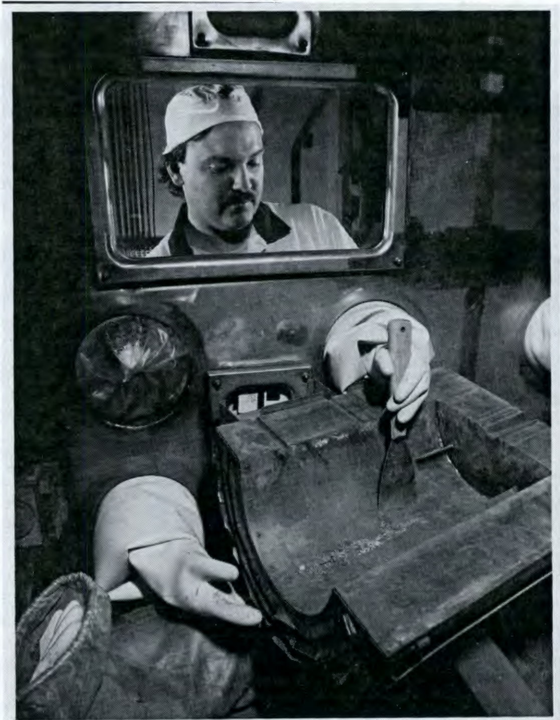
Figure 22. Nuclear Operator Removes Residual Plutonium Contamination from Equipment Inside N Cell Glove Box, as Part of Deactivation, Early 1996.
