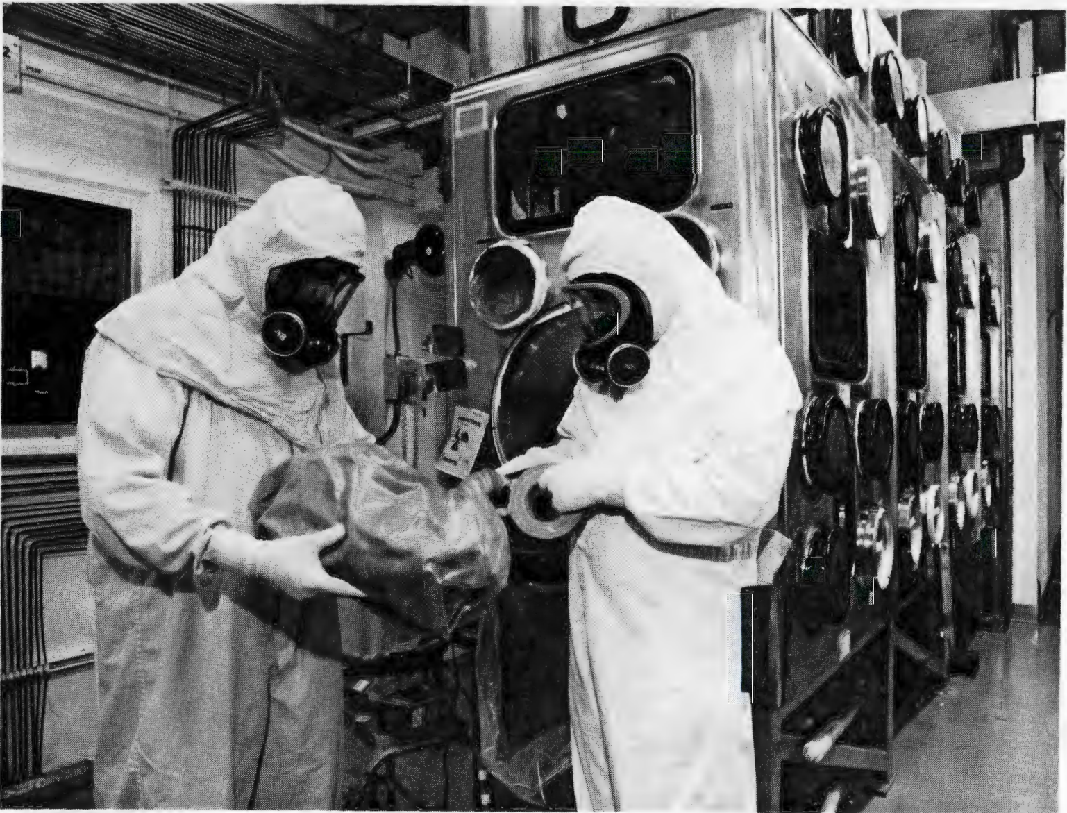
Figure 24. N Cell Equipment is Sealed Shut After Cleanout, PUREX, 1996.
