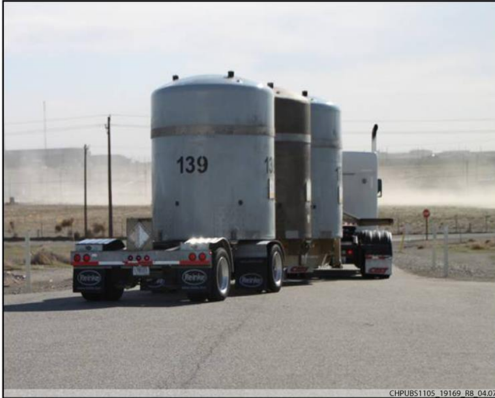
Figure 5-3. TRUPACT-II Shipment of TRUM Waste to WIPP
