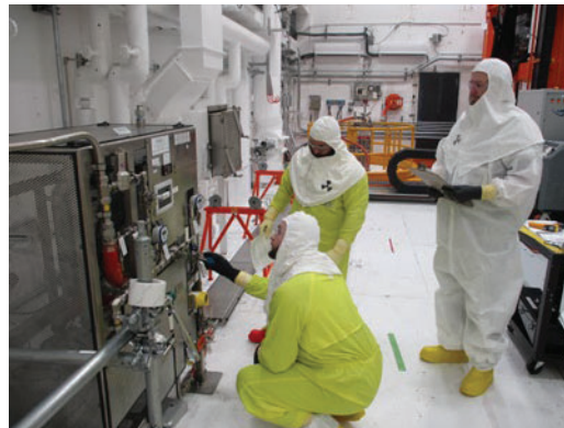
Team performing Evacuation and Helium Backfill of CSS in WESF Canyon
